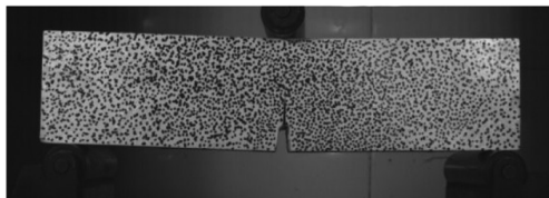
Figure 11. Reference image in the three-point bending test
